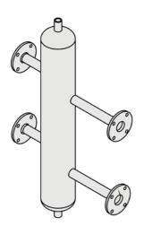
These are used to compensate the pressure differences in systems where multiple pumps and / or heating circuits are used, to eliminate excessive pressure differences between boiler's inlet and outlet water temperatures and to prevent thermal stresses in the boiler.
