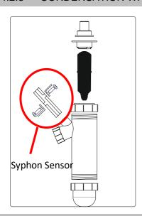
Condensation water which is generated during to the combustion, transfers to the water drain connection by the syphon and drain hose.
