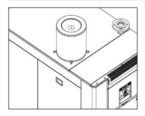
If **SUPERBOX** boilers will be used in to a dirty air environment, they must be supported with the air inlet filters. This optional filter must be checked regularly.
