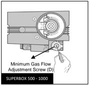
Minimum load emission setting is done by measuring the CO2 value in the flue gas. The following steps should be followed for this instant measurement on a boiler operating at minimum capacity.
