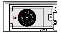
**SUPERBOX** boilers are equipped with Gas Pressure Switch as a measure against high gas pressure. This value is adjusted to **40 mbar**. In cases where the mains pressure is higher than the set value, the gas pass is stopped and 132 (Safety Shutdown of Gas Processor) error code will be displayed on the control panel. This error code can only be reset by performing a reset operation.
