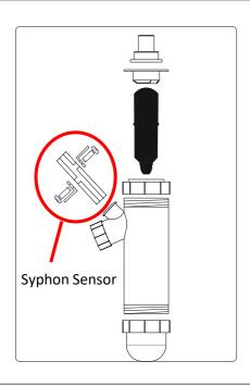
Condensation water which is generated during to the combustion, transfers to the water drain connection by the syphon and drain hose.
