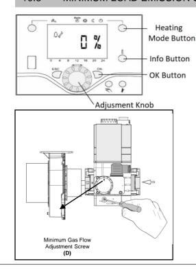
Minimum load emission setting is done by measuring the CO2 value in the flue gas. The following steps should be followed for this instant measurement on a boiler operating at minimum capacity.
