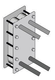
Plate heat exchangers are hydraulic equipments that separates the boiler and the installation (primary and secondary zones). Unlike the hydraulic separator circulating water in the plate heat exchanger never interfere with the water goes through the boiler and the water goes through the installation. Only heat transfer occurs here. Preferred for many purposes;
