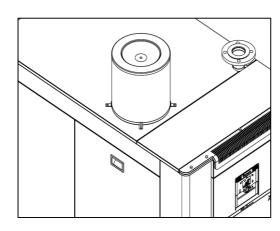
If **ALUBOX** boilers will be used in to a dirty air environment, they must be supported with the air inlet filters. This optional filter must be checked regularly.
