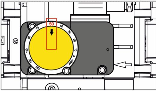
**Alubox** boilers are equipped with a Gas Pressure Switch as a measure against high gas pressure. This value is adjusted to **50 mbar**. In cases where the mains pressure is higher than the set value, the gas pass is stopped and 132 (Gas pressure switch safety shut-down) error code will be displayed on the control panel. This error code can only be reset by performing a reset operation.
