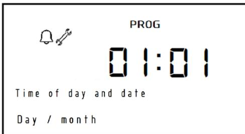
Push **OK** button for adjustment. Push **OK** button to adjust hour and minute settings.
