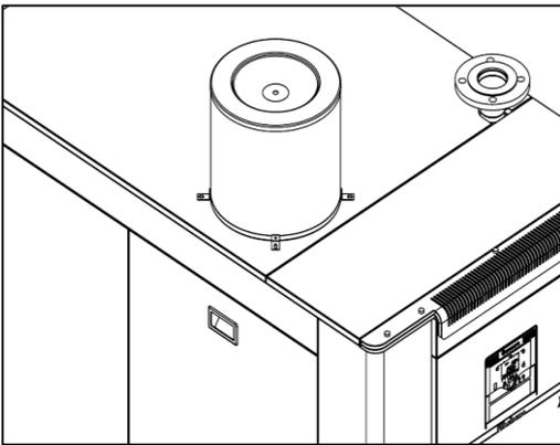
If **ALUBOX** boilers will be used in to a dirty air environment, they must be supported with the air inlet filters. This optional filter must be checked regularly.
