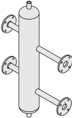
These are used to compensate the pressure differences in systems where multiple pumps and / or heating circuits are used, to eliminate excessive pressure differences between boiler's inlet and outlet water temperatures and to prevent thermal stresses in the boiler.
