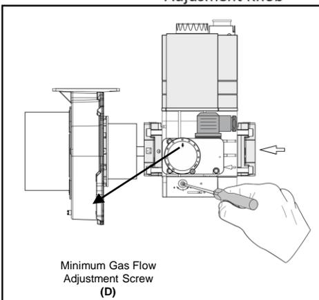
Minimum load emission setting is done by measuring the CO<sub>2</sub> value in the flue gas. The following steps should be followed for this instant measurement on a boiler operating at minimum capacity.
