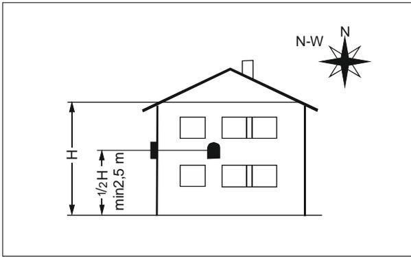
When an outside temperature sensor installed, boiler will adjust supply temperature according to the outside temperature in order to provide energy saving without compromise the comfort.
