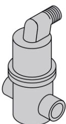
**ALUBOX** boilers have an automatic relief valve for the evacuation of the air accumulated in the heat exchanger. However, for the evacuation of the air that may occur in the installation, it is necessary to place one or more automatic air relief valves in the appropriate places of the installation. Local regulations must be followed in this regard.
