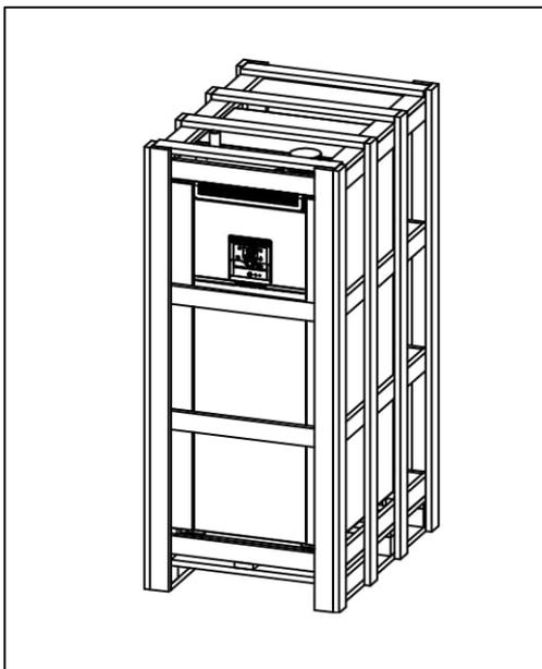
**ALUBOX** boilers are shipped on pallets as they are completely assembled, tested and protected against damage by wooden frame and nylon.
