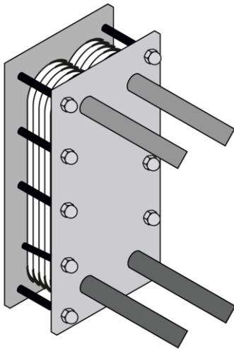
Plate heat exchangers are hydraulic equipments that separates the boiler and the installation (primary and secondary zones). Unlike the hydraulic separator circulating water in the plate heat exchanger never interfere with the water goes through the boiler and the water goes through the installation. Only heat transfer occurs here.
