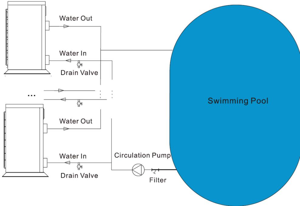
The filter connected with pipes should be cleaned regularly to make sure the water inside systems clean,
