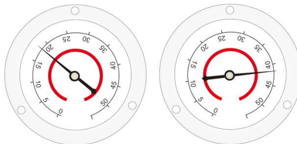
The manometer is a kind of high pressure equipment, when the heat pump is on, the manometer pointer would point to the pressure value of refrigerant, the max. value of protection is 42kg/Cm<sup>2</sup>. When the heat pump is off, the pointer would point to the same value as actual ambient temperature (e.g. 28°C) and related air pressure (e.g. 18kg/ Cm<sup>2</sup> ).
